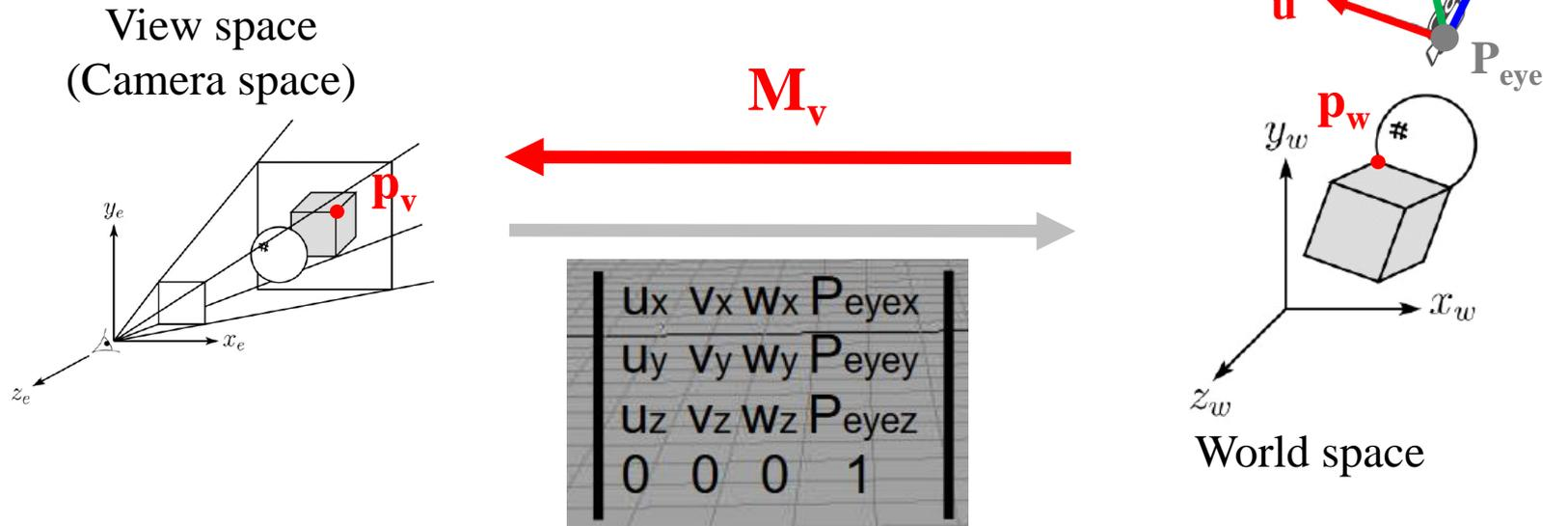
$$M_v = \begin{bmatrix} u_x & v_x & w_x & P_{eyex} \\ u_y & v_y & w_y & P_{eyey} \\ u_z & v_z & w_z & P_{eyez} \\ 0 & 0 & 0 & 1 \end{bmatrix}^{-1} = \begin{bmatrix} u_x & u_y & u_z & -\mathbf{u} \cdot \mathbf{p}_{eye} \\ v_x & v_y & v_z & -\mathbf{v} \cdot \mathbf{p}_{eye} \\ w_x & w_y & w_z & -\mathbf{w} \cdot \mathbf{p}_{eye} \\ 0 & 0 & 0 & 1 \end{bmatrix}$$
