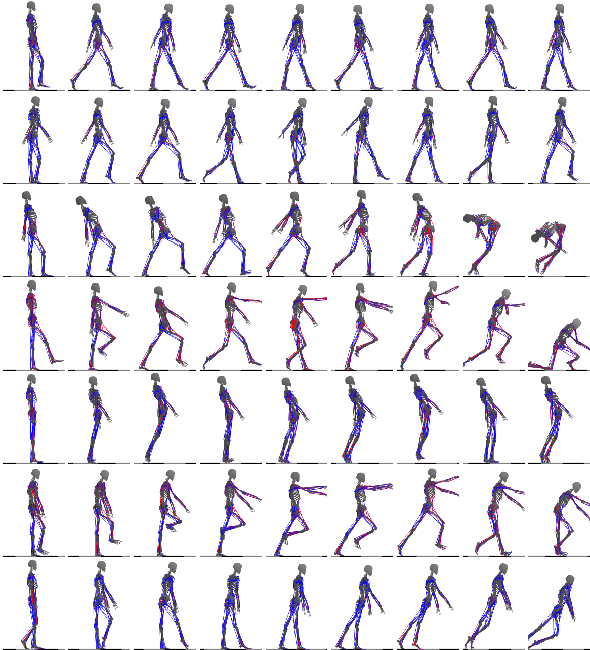
Figure 1: Experimental results. From top to bottom: Ours (row 1), Dense energy (MET) only (row 2), Sparse energy (CoT) only (row 3), Without energy reward (row 4), Start with a double stance pose (row 5), Dense activation reward (row 6), Without muscle fiber length in observation (row 7)
